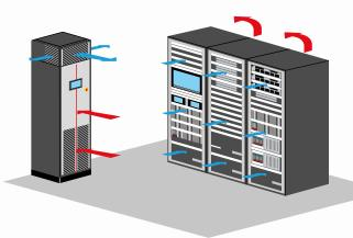
TYPICAL INSTALLATION: DATA CENTERS WITH OR WITHOUT RAISED FLOOR
