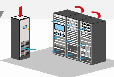
TYPICAL INSTALLATION: DATA CENTER WITHOUT RAISED FLOOR
