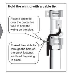
Insert the flow sensor into the couplers, and then fit the quick fasteners where the flow sensor and the couplers are connected to each other. Keep the guick fasteners out of contact with the wiring so as not to damage the wiring. Hold the wiring to the quick fastener with a (short) cable tie as shown in the figure to keep the wiring from being damaged.
