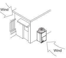
• Install the outdoor unit in a place where it is not exposed to direct wind, such as behind a building.
