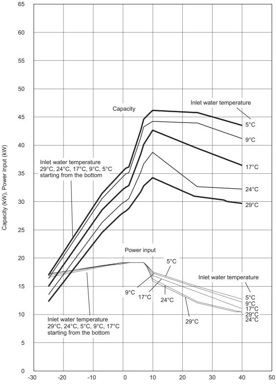
Outlet water temperature 60~70°C Energy saving operation 2 mode
