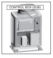
(2) Thread the wiring into the unit.
