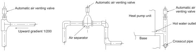
Air venting valve installation example
