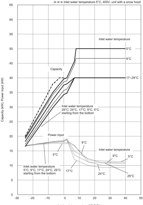
Outlet water temperature 80°C Energy saving operation 2 mode
