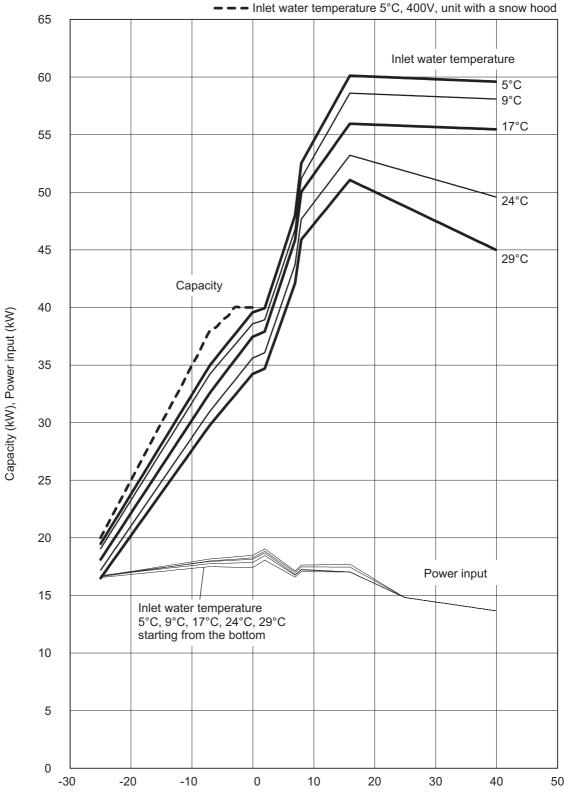
Outlet water temperature 80°C Max capacity operation mode
