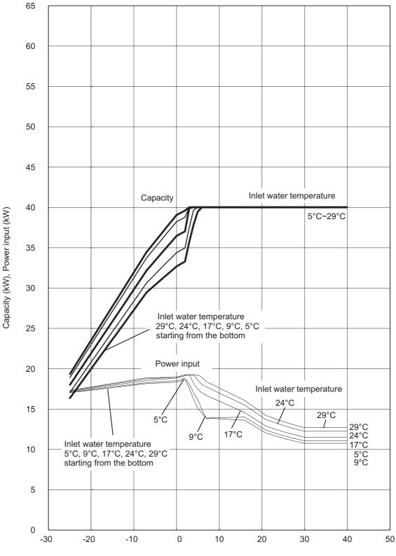
Outlet water temperature 90°C Energy saving operation 1 mode
