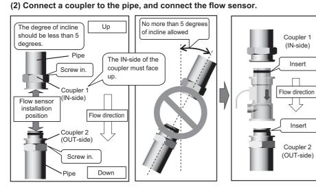
Attach the coupler to the pipe so that the IN-side of the coupler faces up and the OUT-side of the coupler faces down. (Water flows from top to bottom.) The incline of the pipe should not exceed 5 degrees. Keep the sensor away from water. The flow sensor is 71.5 mm long. Keep an appropriate distance between the couplers. Fit the flow sensor to the coupler.
