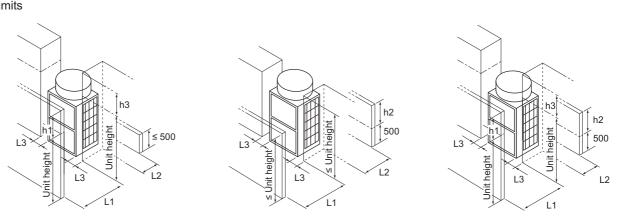
Add the dimension that exceeds the height limit (shown as "h1" through "h3" in the figures) to L1, L2, and L3 as shown in the table below.
