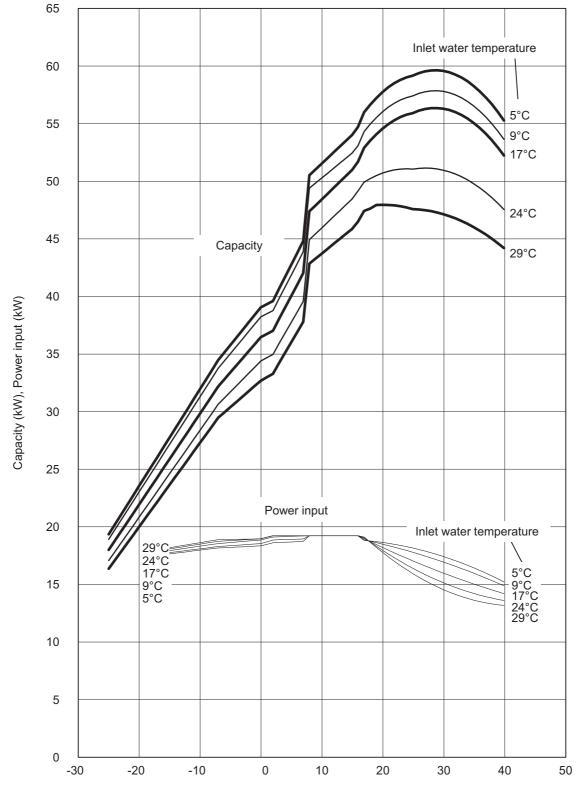
Outlet water temperature 90°C Max capacity operation mode
